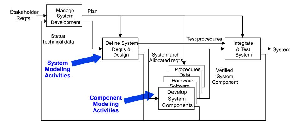
Integrated Product Development (IPD) is essential to improve communications A Recursive V process that can be applied to multiple levels of the system hierarchy
