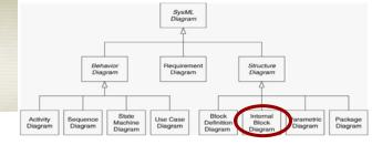
Represents interconnection and interfaces between the parts of a block
