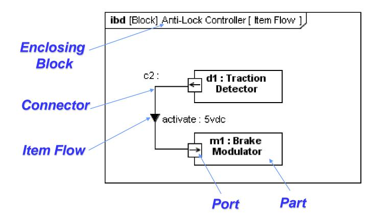
Internal Block Diagram Specifies Interconnection of Parts
